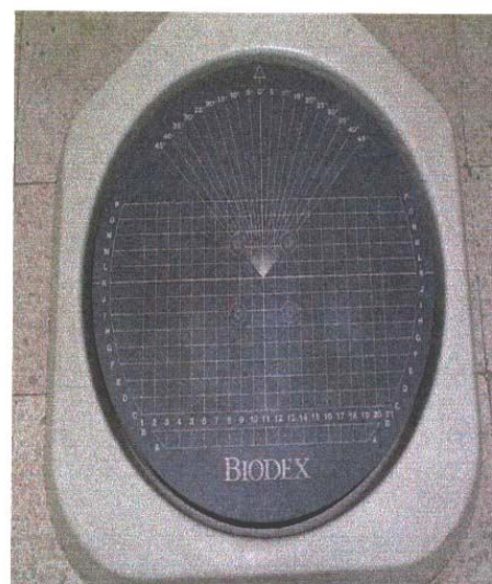
Fig. (2): Biodex platform coordinates grid mesh to identify foot coordinates and angles.
