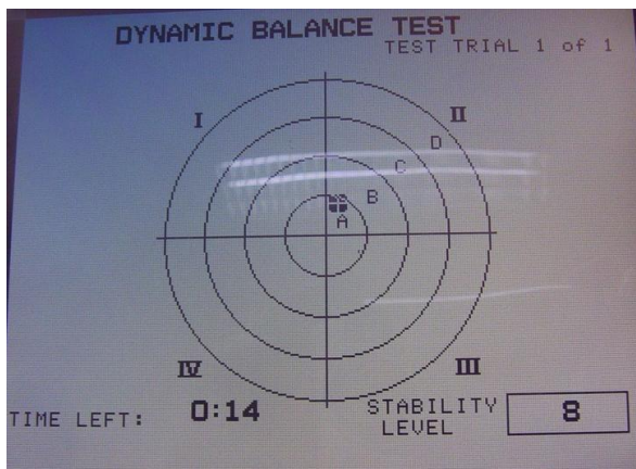
Fig. (3): Balance test screen that consisted of four quadrants and four intrinsic circular zones, where the cursor in the inner most indicated the higher stability.
