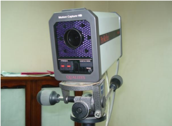
Fig. (1): The motion capture unit (high speed camera).
