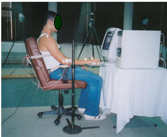
Fig. (3): The subject while performing the task at a zero slope mouse platform. The EMG activity is recorded from the wrist flexors and extensors.
