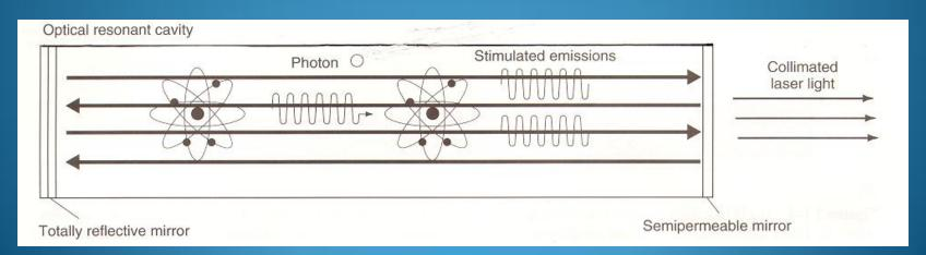
✓ Eventually so many photons are stimulated that the chamber cannot contain energy and photons of a particular wavelength are ejected through the semipermeable mirror producing amplified light through stimulated emissions.
