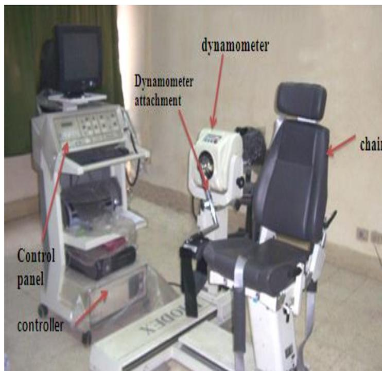
**Fig.(1):** Biodex system 3 Isokinetic dynamometer.
